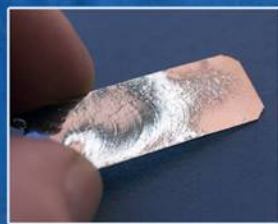
Rhenium Metal Sheet produced by rapid infrared melting (melting point 3450°K) of a powder compact
