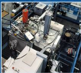
Electron-beam Melting Furnace for purification and alloying of refractory metals
