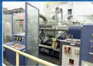
1200 Ton Extrusion Press with preheat to 2000°C for refractory metals and alloys
