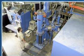
Vacuum Arc Remelt Furnace used for tungsten, molybdenum, niobium, iridium, and other refractory metal alloys
